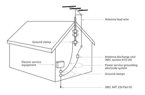
FIGURE 1. Example of Antenna Grounding
